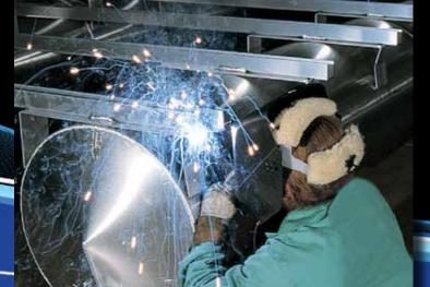
OUR PONTOONS ARE HAND WELDED TO CROSS-MEMBERS OF 1/4" THICK ALUMINUM. THERE ARE NO NUTS THAT CAN BECOME LOOSE OR BE LOST, ASSURING YOU OF GREATER PEACE OF MIND WHILE ON THE WATER.
